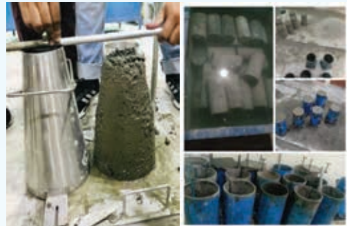
Concrete cylinders preparation, workability testing and curing
