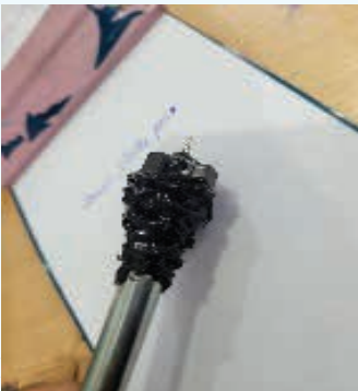
Prototype Pen Designed with Magnetic Stabilization to Assist Individuals with Hand Tremors Regain Writing Control
