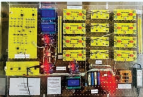
Hardware implementation of hybrid balancer for lithium-ion batteries
